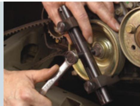
**Multi-diameter damper pulley puller****DM.50**
