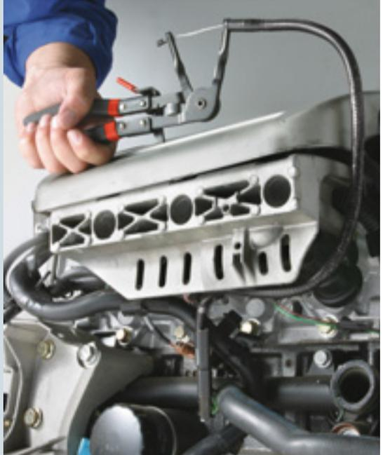
**Spring clamp fitting and removal tool**
