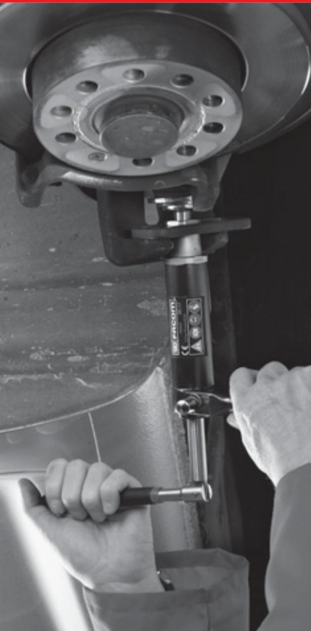
*Essential for replacing brake pads.*
